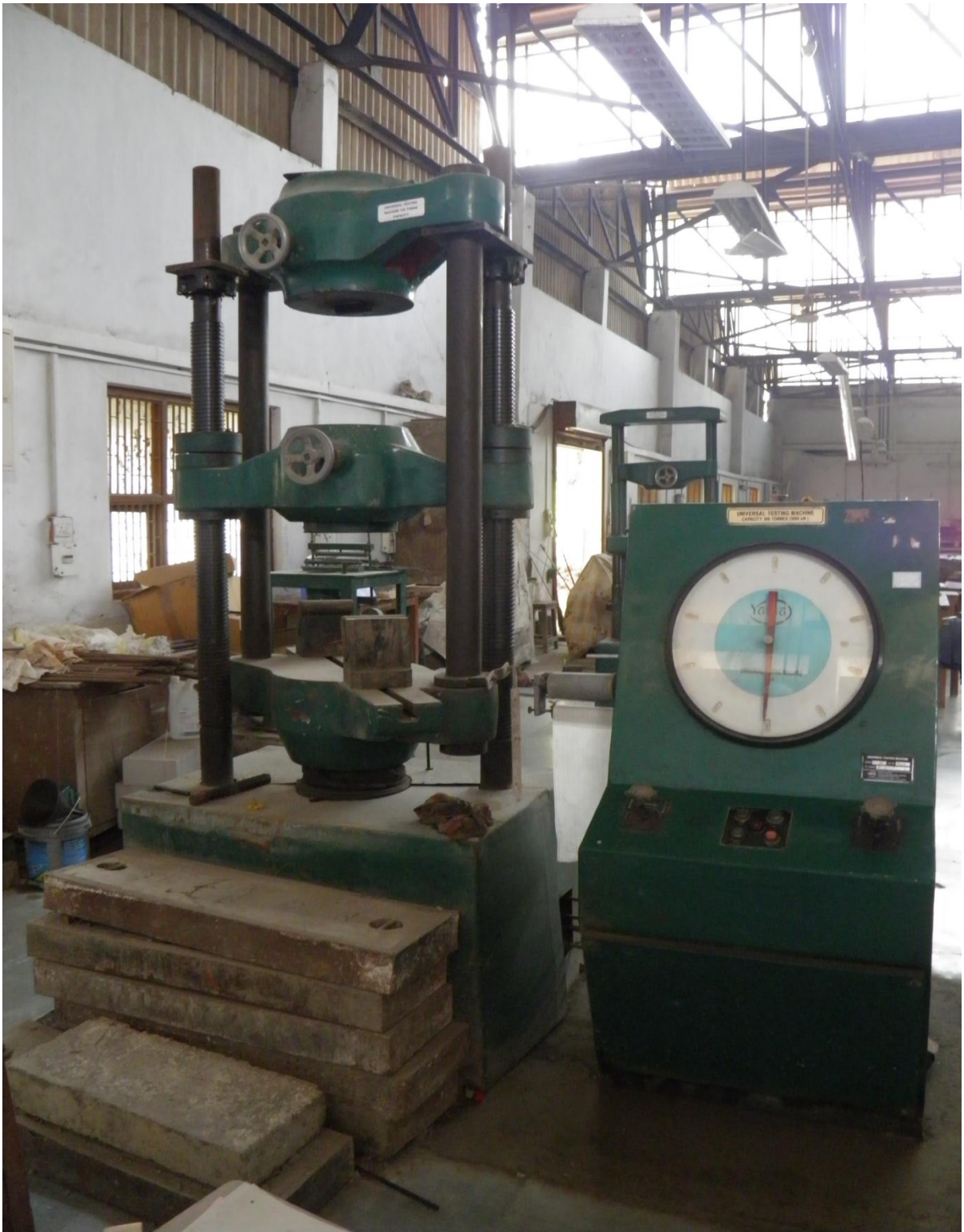
UTM- capacity 40 tonne
