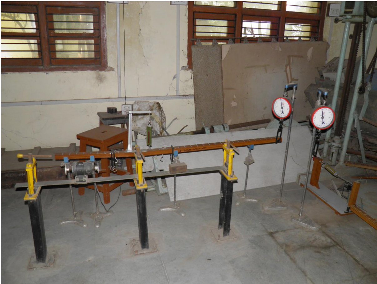
Two span supported model
