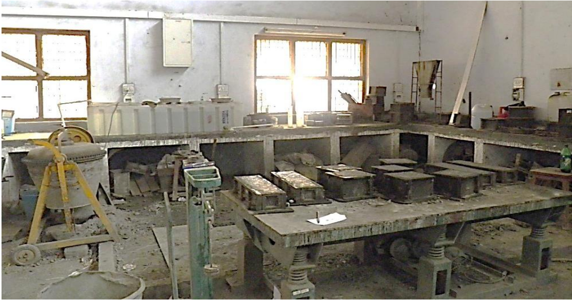
Vibration table and casting yard
