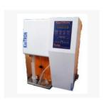
**Nitrogen Analyzer** used for the detection of nitrogen in liquid or organic samples.
