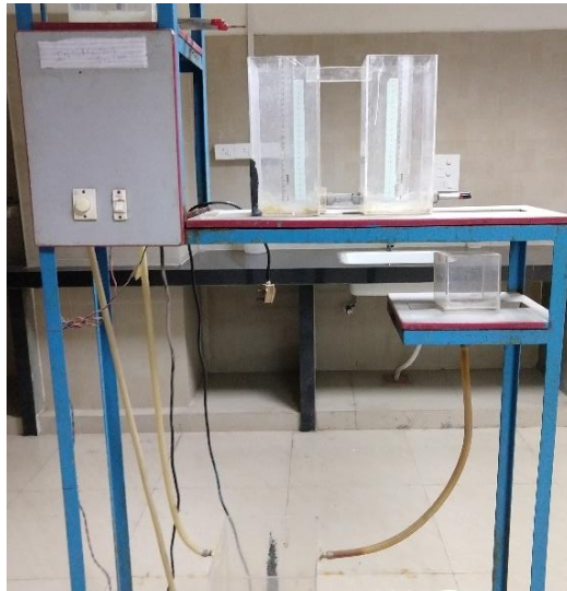
4. Second Order System (Interacting Tanks)
