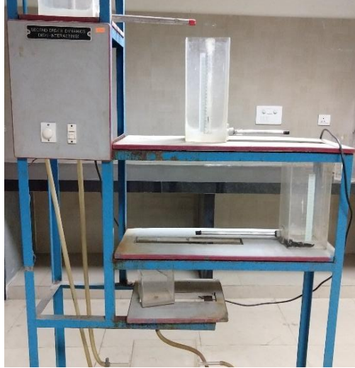
4. Second Order System (Interacting Tanks)
